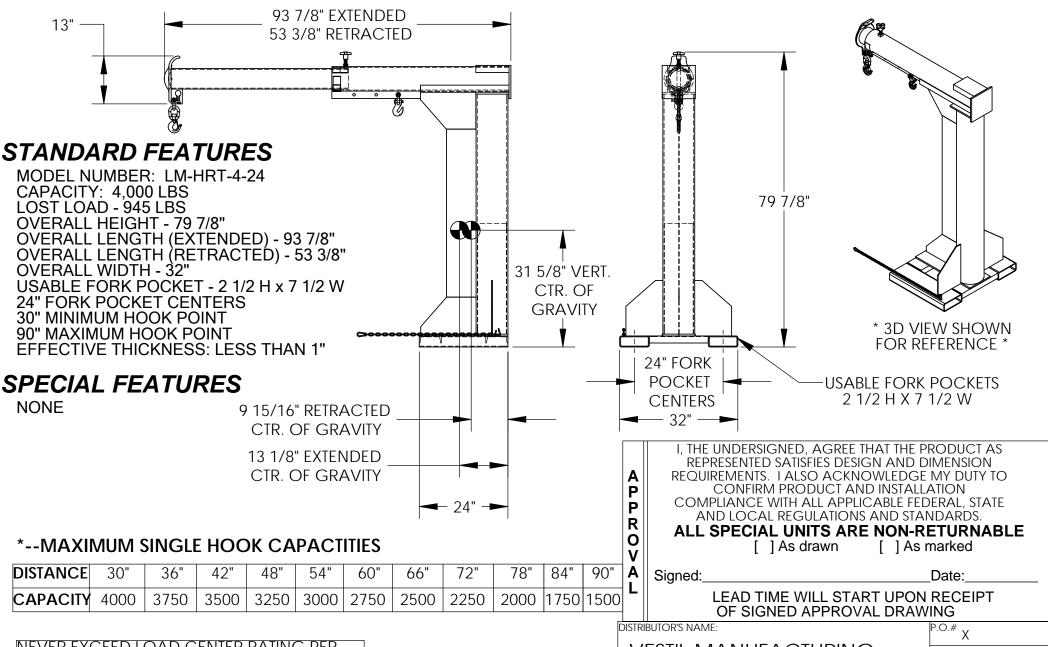
NEVER EXCEED LOAD CENTER RATING PER FORK TRUCK MANUFACTURER'S GUIDELINES. DO NOT USE THIS FORK TRUCK ATTACHEMENT IF LOAD WILL EXCEED FORK TRUCK MANUFACTURER'S LOAD CENTER RATING.
