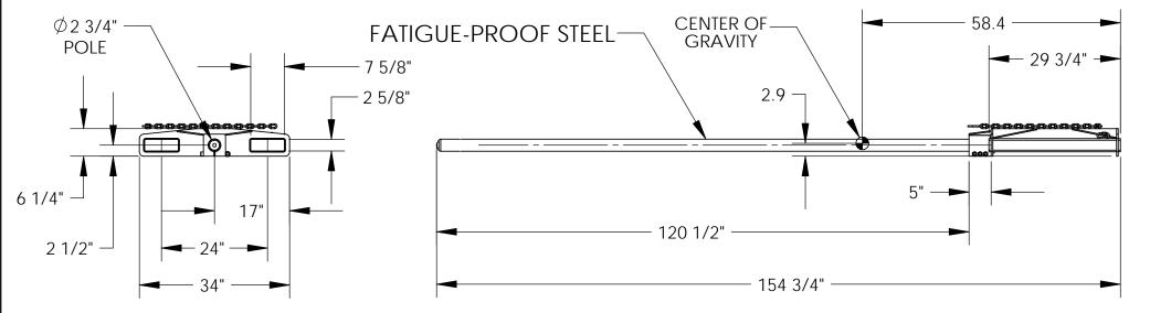
HORIZONTAL CENTER OF GRAVITY: 58.4" VERTICAL CENTER OF GRAVITY: 2.9 LOST LOAD: 380 LBS. (APPROX.)
