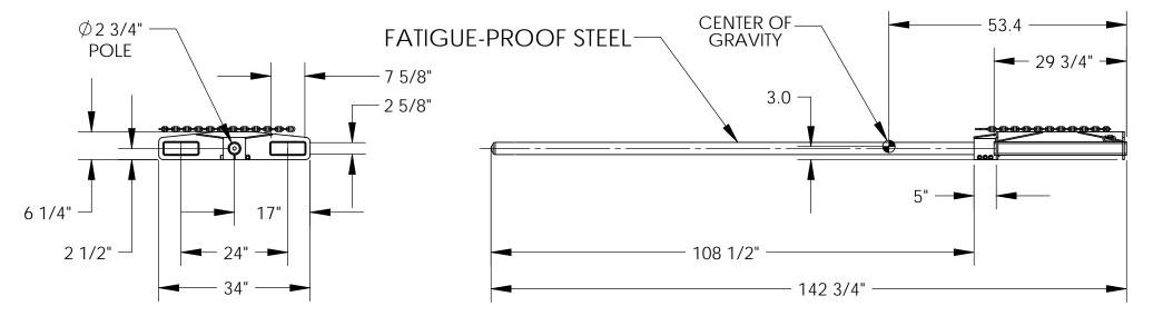
HORIZONTAL CENTER OF GRAVITY: 53.4" VERTICAL CENTER OF GRAVITY: 3.0" LOST LOAD: 360 LBS. (APPROX.)
