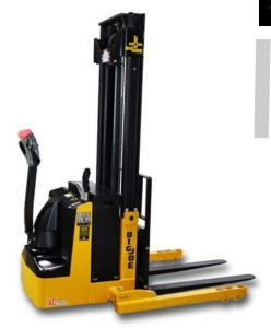
Reduced travel speed when forks are above 12" fork height. Neutral braking-antiroll back on ramps.
