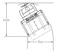
Note: Aisle dimensions listed above assume the bay width to be straddle OD plus 2" (1" on each either side of straddle leg). Straddle OD is the load width plus 8"
