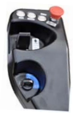
Travel, Lift, Lower, Key Switch and EPD Controls
